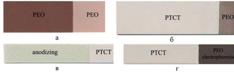
Figure 2. The appearance of coatings obtained on bars of aluminium based alloys with plasma electrochemical method: (a), (b), (d) – 2024; (c) – 4L33.
